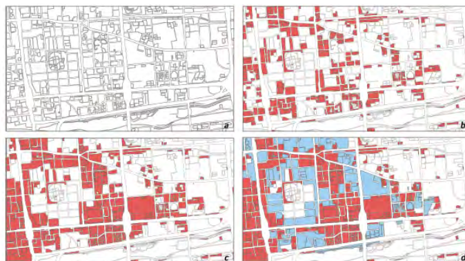
Figure 3 The interaction maps to select urban blocks at t and t+1 time: (A) the initial blocks enclosed by urban streets; (B) identification of initial urban blocks (in red); (C) captured urban blocks at t time (in red); (D) selection of new urban blocks at t+1 time (in blue). (Color figure available online.)
