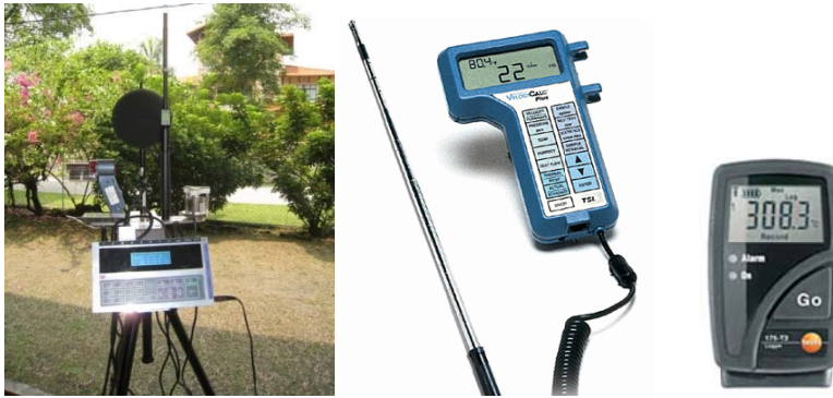
Figure 1. Babuc A (left), mobile TSI VelociCalc Plus Meters (middle), and Electronic Mini Thermohygrograph (right)
