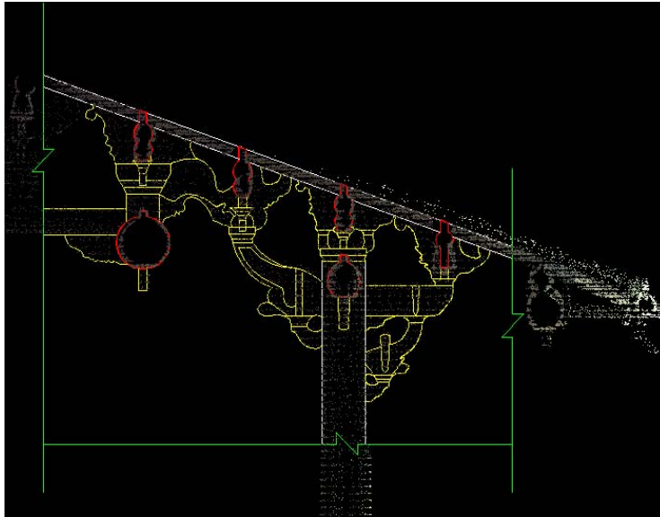
Figure 12. The drawing of the Dougong beams above the Gold Pillar using the cloud of points
