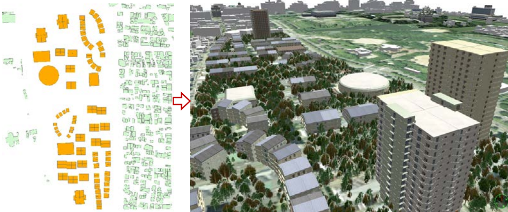
Figure 6. Proposed layout for the town and an automatically generated 3D urban model: low density in the middle area for condominiums with green spaces and urban facilities, and high density in both side areas for official housing and public housing
