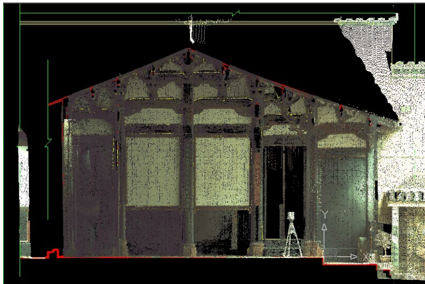
Figure 6. The drawing of the entrance profile section from the cloud of points
