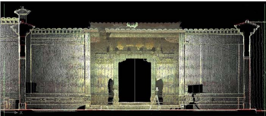
Figure 5. The drawing of the entrance vertical face section from the cloud of points
